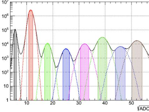
**Fig. 3:** A typical n-side truncated mean distribution in units of  $\sqrt{ADC}$ . The peaks of nuclei up to oxygen are clearly visible. The super-imposed gaussian functions are constructed from the parameters resulting from a multi-gaussian fit to the distribution.
