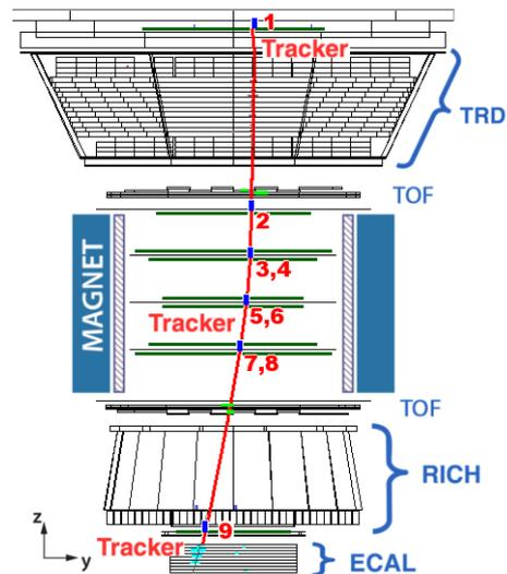
**Fig. 1:** The figure displays the main sub-detectors composing AMS-02, presented in the bending ( $y-z$ ) plane. The red line corresponds to a measured low energy proton.
