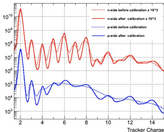
**Fig. 5:** Overall improvement in the tracker charge measurement after applying the calibration, for the n-side (red) and p-side (blue) measurements. The effect is shown up to silicon ( $Z=14$ ) where the n-side saturation starts degrading the measurement.
