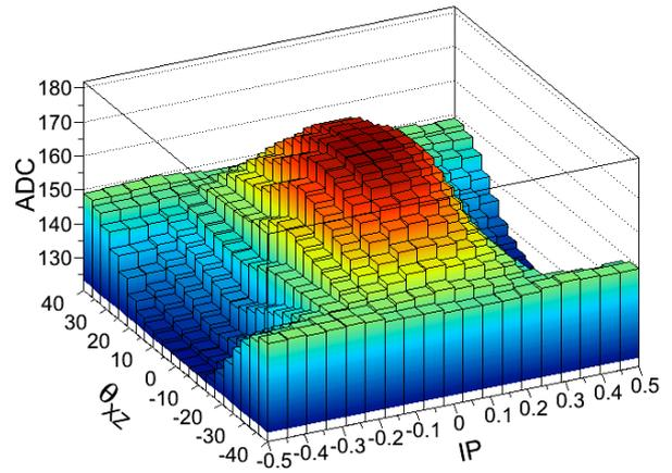
**Fig. 2:** Illustration of the dependence of the raw signal on the impact position of the particle and its inclination for a selected sample of helium nuclei. The maximum of collection efficiency appears when the particle traverses at vertical incidence, impinging directly on a readout strip, i.e.  $IP = 0$  and  $\theta_{XZ} = 0$ .
