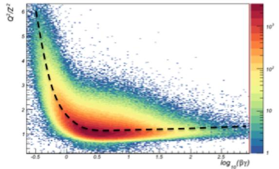
**Fig. 4:** Energy dependence of the proton energy loss in the silicon tracker.
