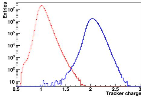
**Fig. 1:** Tracker charge distributions of proton and Helium pure sample selected by an independent charge measurement by TOF.
