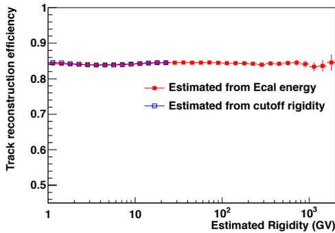
**Fig. 3:** Track reconstruction efficiency estimated from the preselection sample and TOF charge selection, which includes the events passing out of the tracker sensitive area (about 91 %). Red squares: The efficiency as a function of rigidity estimated by Ecal energy deposition. Blue open squares: The efficiency as a function of cutoff rigidity.
