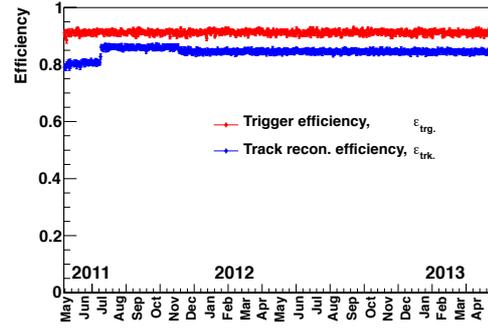
**Fig. 4:** Daily variation of the trigger efficiency ( $\epsilon_{\text{trg.}}$ ), and the proton track efficiency ( $\epsilon_{\text{trk.}}$ ) for rigidities above 20 GV.
