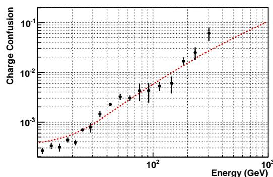
**Fig. 4:** Charge confusion for electron events as function of electron total energy measured in the ECAL. Red line: charge confusion as observed in the simulation. Black points: charge confusion on ISS data as estimated with the Tracker BDT.
