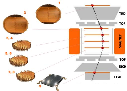
**Fig. 1:** Schematic view of the AMS-02 detector. With pictures of the Silicon tracker layers from 1 to 9.
