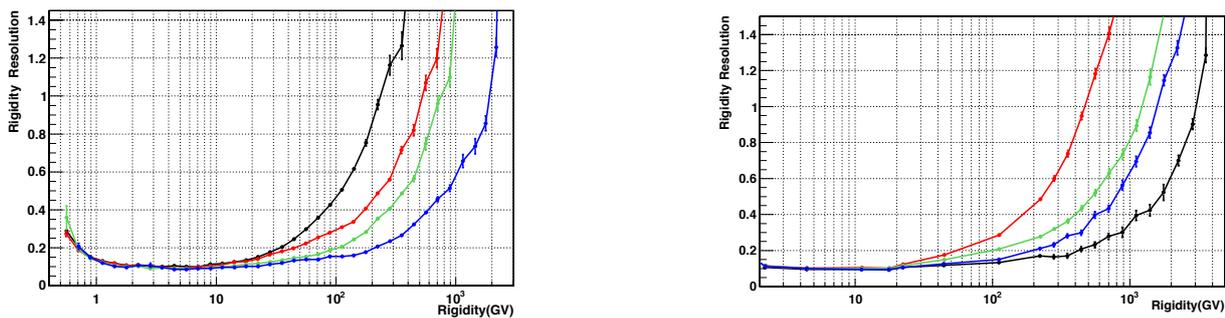
**Fig. 3:** Tracker rigidity resolution for protons(left) and Helium(right) as estimated from the Monte Carlo simulation. The four curves represent the tracker different spans. Black open circles: inner tracker, red full squares: layer1, green open squares: layer9 and blue full circles: layers 1 and 9.
